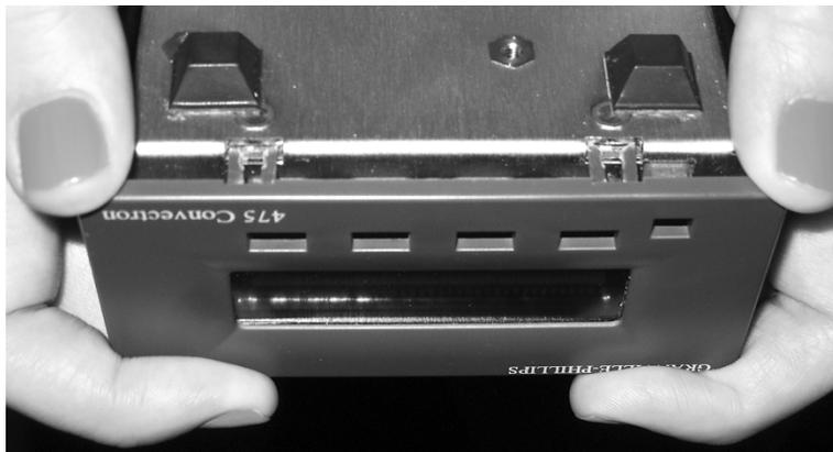
3. Insert the Controller through the front of the panel.
