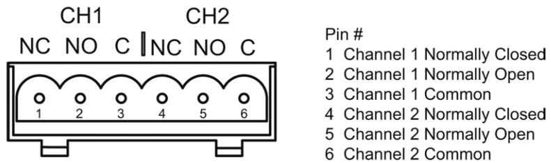
**Figure 2-14 Analog Output Connector (socket)**
