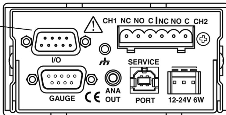
A mating 9-pin D type connector is supplied in the hardware kit. Use shielded cable to minimize electromagnetic radiation or susceptibility. Ground the shield to the metal connector shell or to Pin 5. Do not connect the shield to Pin 7.
