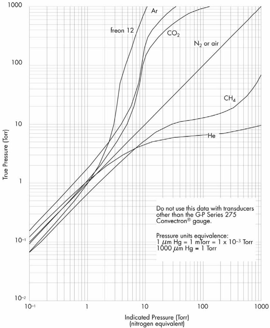
Figure 3-7 Convectron Gauge Indicated vs. True Pressure Curve; .01 to 1000 Torr
