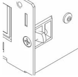
4. Use a Phillips head screwdriver to rotate the Pawl Screw to lock the Controller to the panel. See Figure 2-6.
