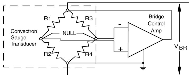
The Convectron gauge operates like a standard Pirani gauge, which employs the principle of a Wheatstone bridge to convert pressure to voltage, but uses convection cooling to enable accurate pressure measurement, when properly calibrated, from  $10^{-4}$  to 1000 Torr. The sensing wire is an ultra-fine strand of gold-plated tungsten or solid platinum.
