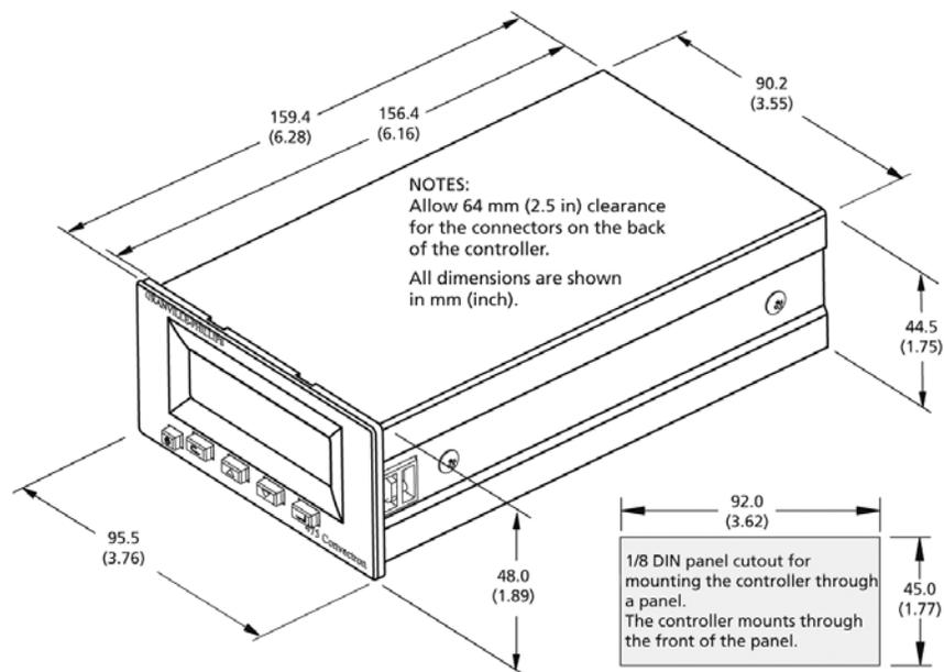
The Controller may be free-standing or panel-mounted. For free standing (benchtop) use, install the provided self-adhesive rubber feet on the bottom of the controller.
