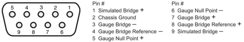
**Figure 2-13 2-Channel Process Control Connector (pins)**
