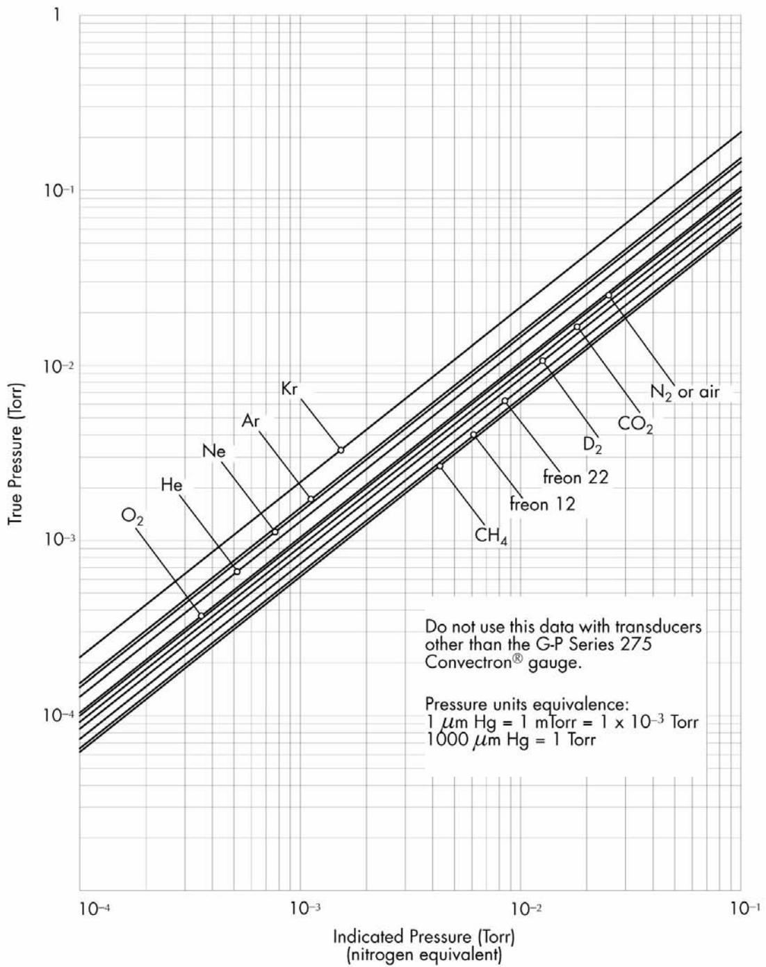
Figure 3-6 Convectron Gauge Indicated vs. True Pressure Curve; .01 to 1000 Torr
