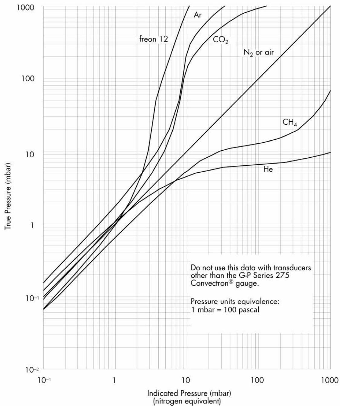
Figure 3-10 Convectron Gauge Indicated vs. True Pressure Curve; .01 to 1000 mbar
