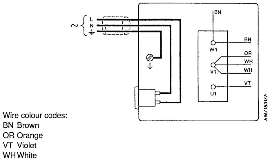
Figure 11 - Electrical supply connection, single-phase motors (high voltage)
