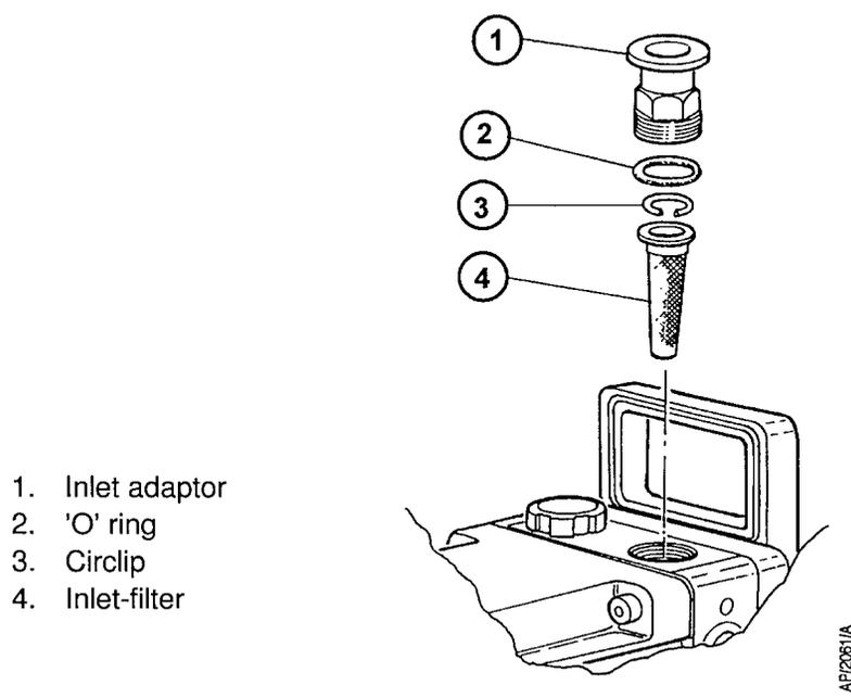
Figure 18 - Inlet-filter removal and replacement (E2M2 illustrated)
