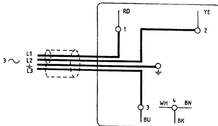
Figure 15 - Electrical supply connection, three-phase motors (high voltage)
