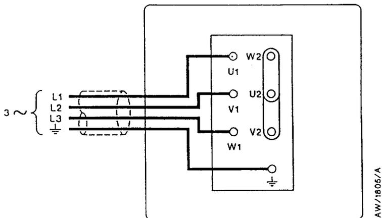
Figure 17 - Electrical supply connection, three-phase motors, ) (high voltage)
