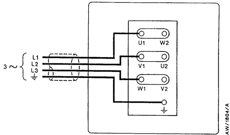
Figure 16 - Electrical supply connection, three-phase motors, (low voltage)
