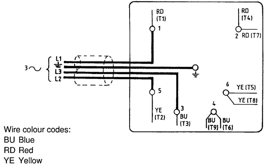
Figure 13 - Electrical supply connection, three-phase motors (high voltage)
