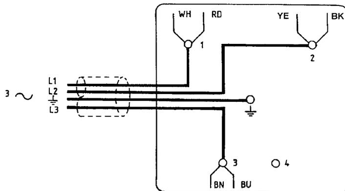
Figure 14 - Electrical supply connection, three-phase motors (low voltage)
