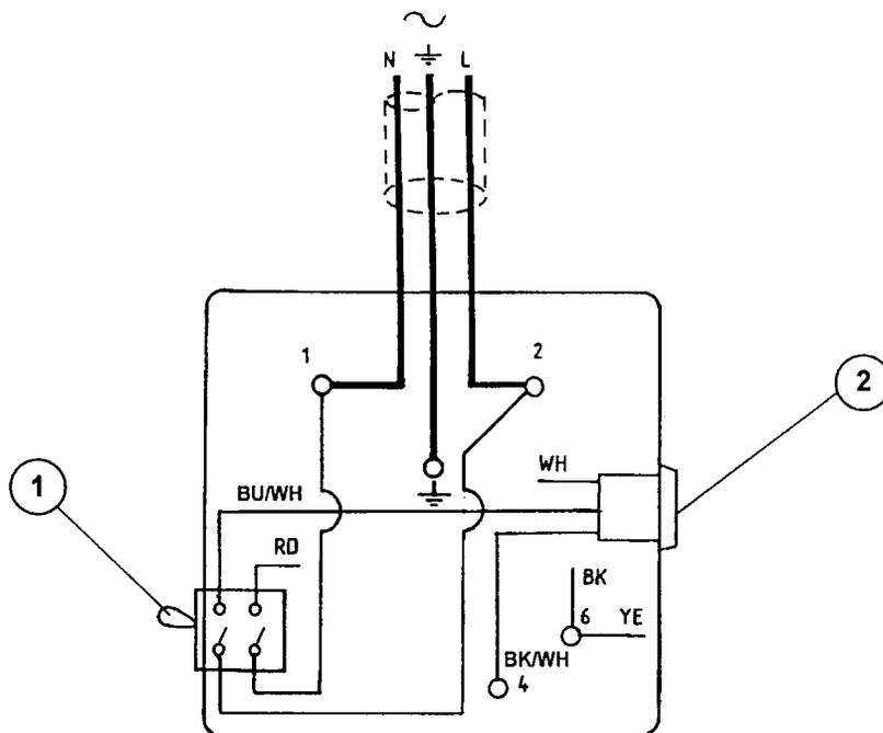
Figure 9 - Electrical supply connection, single-phase motors, (high voltage) (see Table 1 for applicability)
