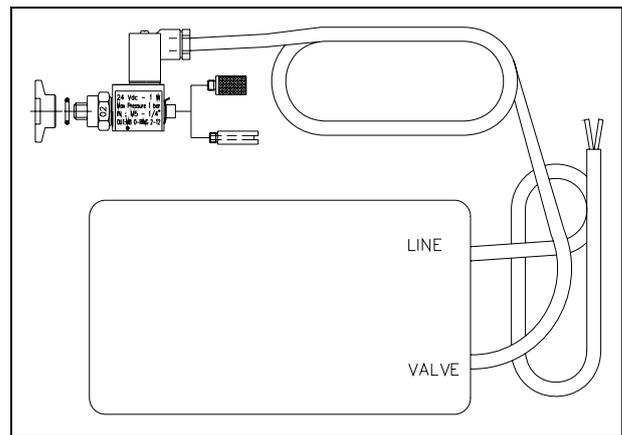
The vent device mod. 969-9831 allows to avoid undesired pump aeration of the pump during a temporary power failure (adjustable time up to 36 min.), and enables an automatic vent operation.
