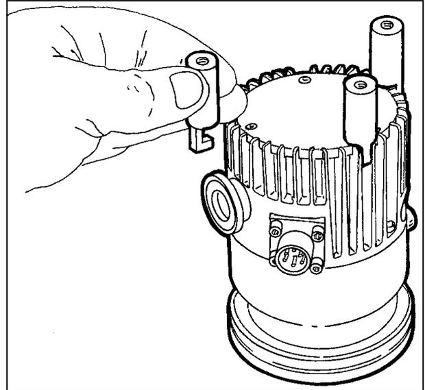
For the feet to the pump by tightening the previously inserted grub screws with the Allen key.
