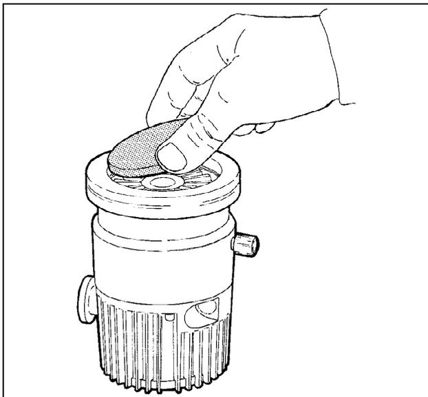
The screen can be mounted on either pump series and is supplied with a small tab for easy removal (see figure).
