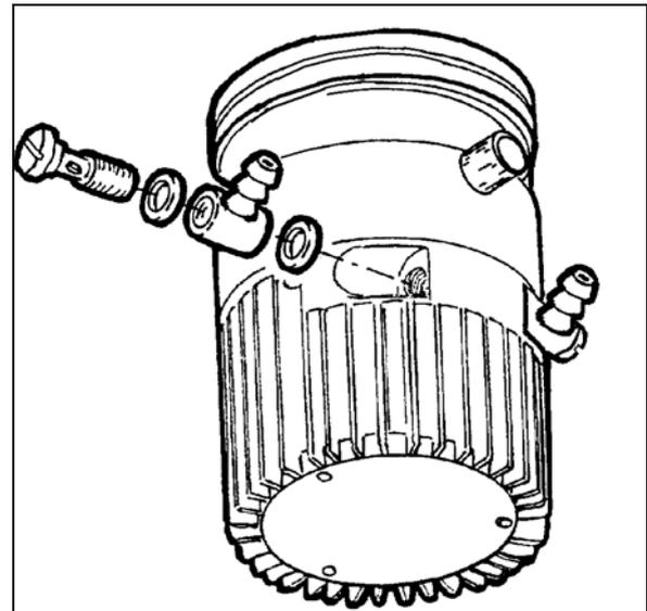
Two 6 mm (1/4") internal diameter rubber or plastic hoses from the water supply must be fitted to the two nozzles.
