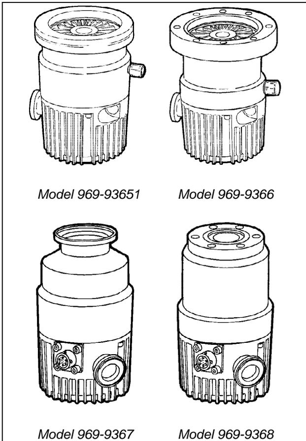
The Turbo-V70LP pump consists of a high frequency motor driving a turbine fitted with 10 bladed stages and 4 Macrotrorr stages. The turbine rotates in an anticlockwise direction when viewed from the high vacuum flange end.
