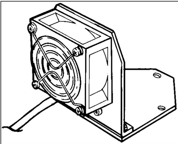
A fan kit model 969-9310 is available for air cooling the pump, when natural air convection is insufficient.
