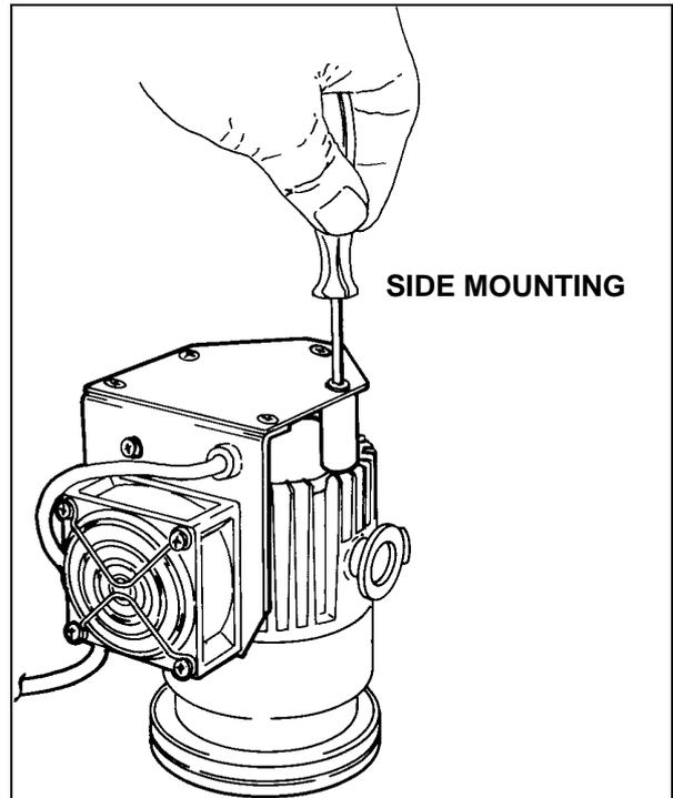
The fan can also be mounted under the pump as shown in the figure.
