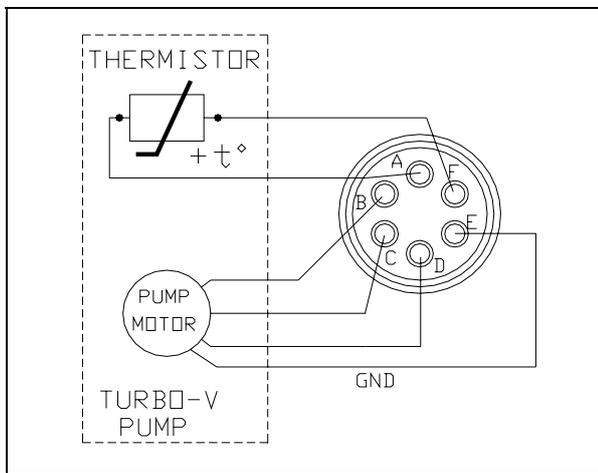
The turbopump is connected to the controller through an 6-pin connector. Pins B, C and D are the 3-phase supply to the motor, pins A and F are connected to the temperature sensor (NTC type, 30 KΩ resistance at 25° C) and pin E is connected to the pump ground.
