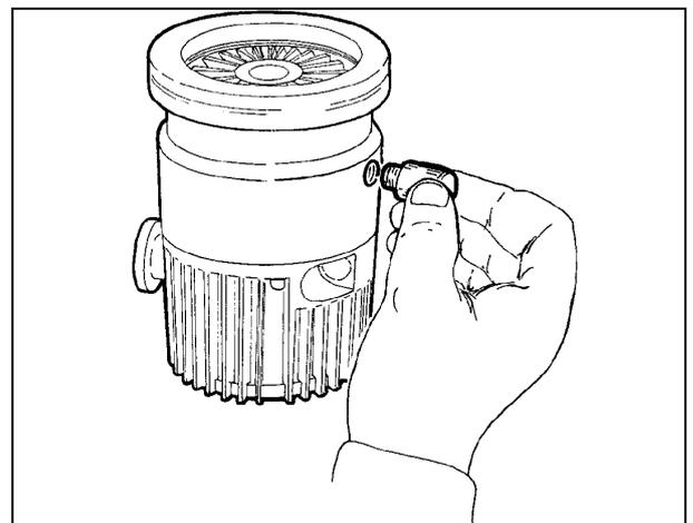
Screw the flange mod. 969-9109 on the pump, taking care of the o-ring right position.
