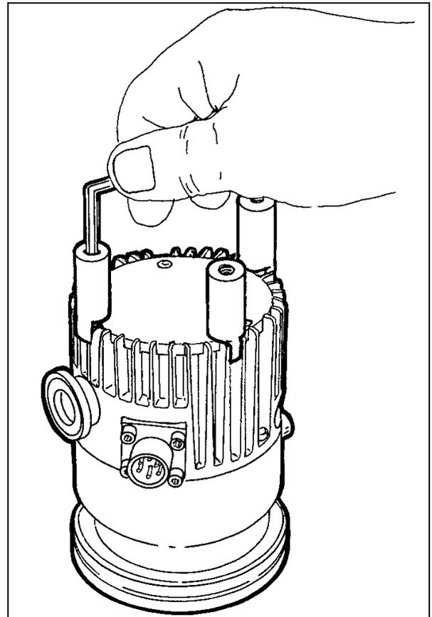
Turn the pump the right way up. Fix the pump to a base by using the three screws provided (M4 thread) in the holes in the three feet.
