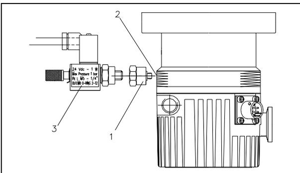
Tighten the valve using a 16 mm hexagonal spanner.
