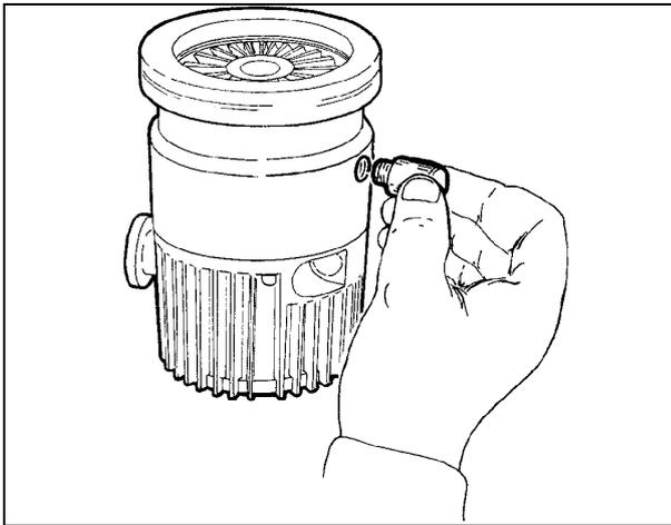
Screw the adapter (1) into the vent hole (2) of the pump.
