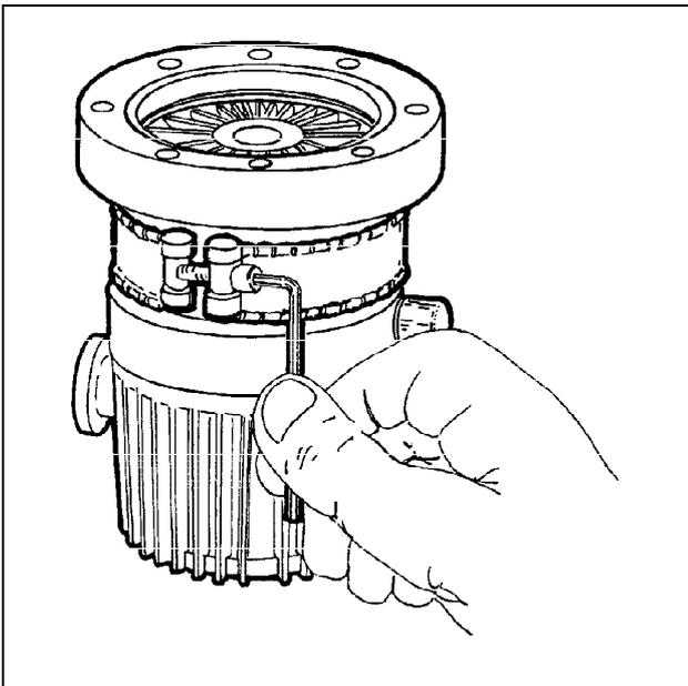
Switch on the heater while the turbopump is in operation. If, for any reason, the turbopump body overheats, it will be automatically cut out by the thermistor sensor.
