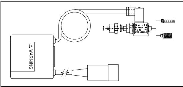
The vent valve mod. 969-9843 enables undesired pump aeration during a temporary power failure (5 sec maximum) to be avoided, and enables an automatic vent operation.
