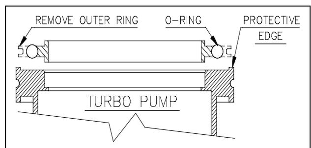
Then fix the two flanges with the clamps or claws as shown in the figure.
