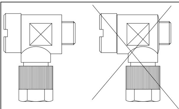
The assembled kit must be screwed into the suitable holes of the pump body with a recommended closing torque of 5 Nm.
