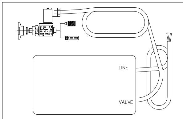
The vent device mod. 969-9831 allows to avoid undesired venting of the pump during a temporary power failure (adjustable time up to 36 min.), and enables an automatic vent operation.
