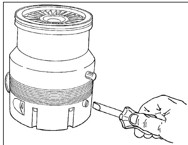
and then screw the gas purge valve (with a torque of 2.5 Nm) as shown in the following figure.
