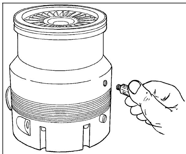
Screw the vent valve into the pump inserting the supplied adapter between the valve and the pump.
