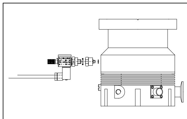
Tighten the valve using a 16 mm. hexagonal spanner with a torque of 2.5 Nm.
