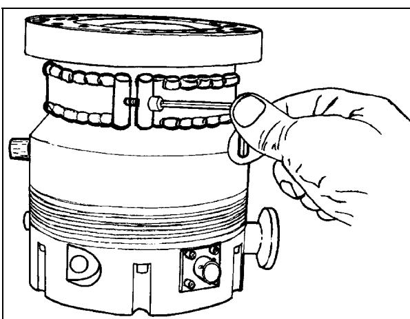
Switch on the heater while the turbopump is in operation. In the event of turbopump overheat, the pump will be automatically cut out by the thermistor sensor.
