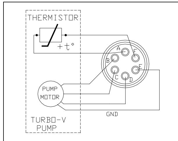
The turbopump is connected to the controller through an 6-pin connector. Pins B, C and D are the 3-phase supply to the motor, pins A and F are connected to the temperature sensor (NTC type, 30 K $\Omega$  resistance at 25° C) and pin E is connected to the pump ground.
