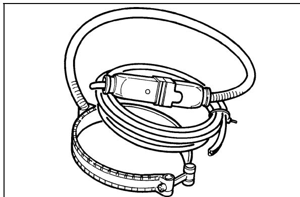
The heater band model 969-9804 and 969-9803 can be used to heat the pump casing when a bakeout is needed.
