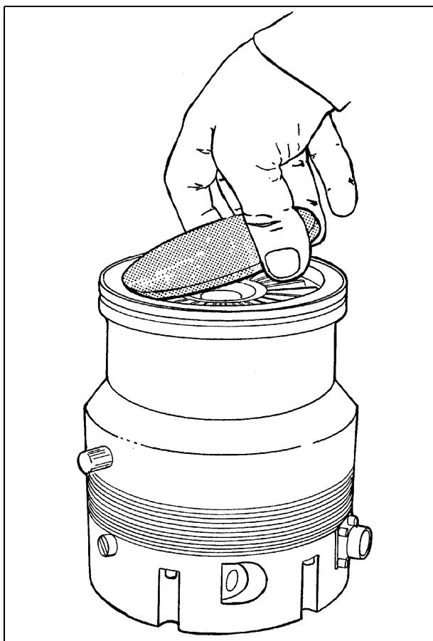
The screen can be mounted on each pump model and is supplied with a small tab for easy removal (see figure).
