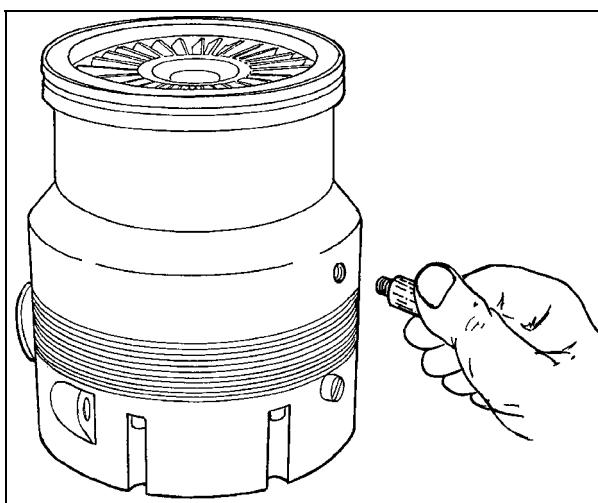
Screw the flange mod. 969-9109 on the pump, taking care of the o-ring right position.
