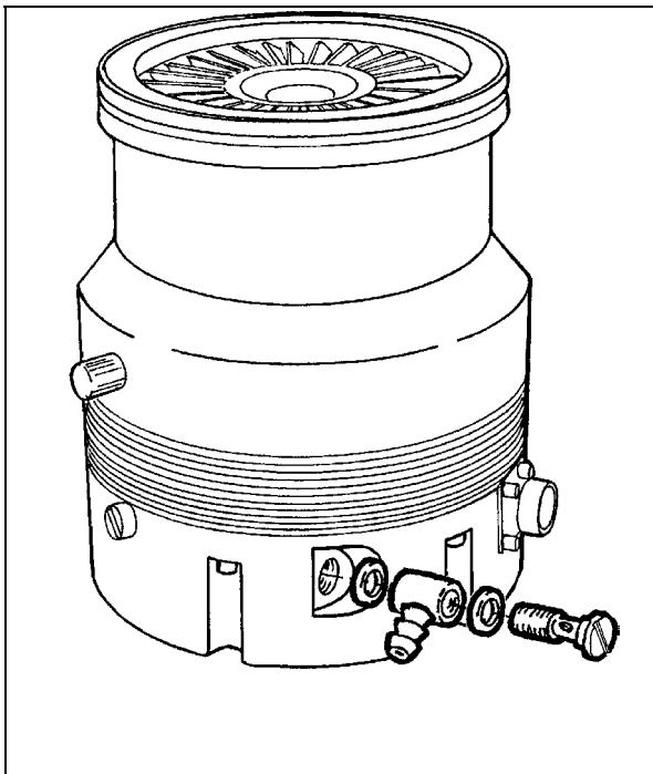
Two 6 mm (1/4") internal diameter rubber or plastic hoses from the water supply must be fitted to the two nozzles.
