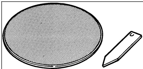
The inlet screens mod. 969-9302 and 969-9303 prevents the blades of the pump from being damaged by debris greater than 0.7 mm diameter.
