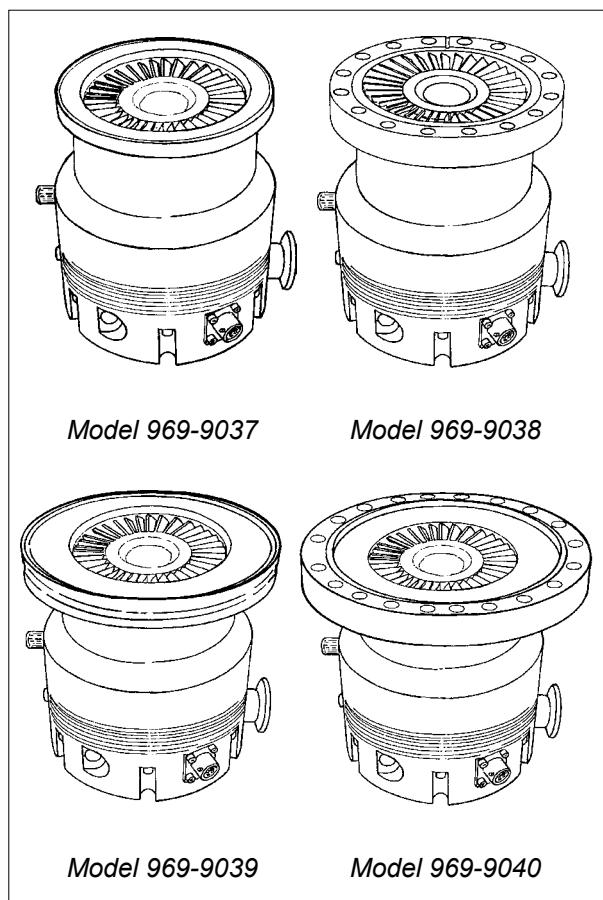
The Turbo-V300HT pump consists of a high frequency motor driving a turbine fitted with 8 bladed stages and 3 Macrotorr stages. The turbine rotates in an anticlockwise direction when viewed from the high vacuum flange end.
