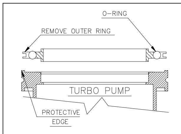
Then fix the two flanges with the clamps or claws as shown in the figure.
