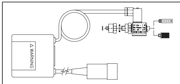
The vent valve mod. 969-9833 allows to avoid undesired venting of the pump during a temporary power failure (5 sec maximum), and enables an automatic vent operation.
