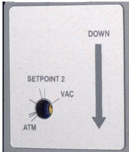
Figure 10 Potentiometer Pressure Markings on the Side Panel
