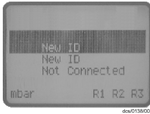
Figure 16 - New gauge connected
