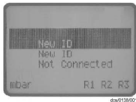
Figure 16 - New gauge connected
