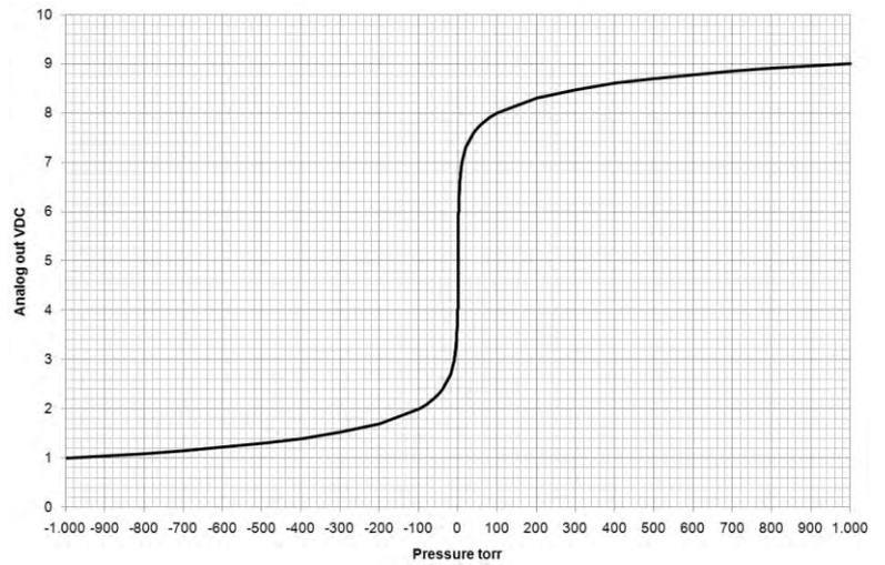
For positive pressure ( $V_{out} > 5V_{dc}$ )
