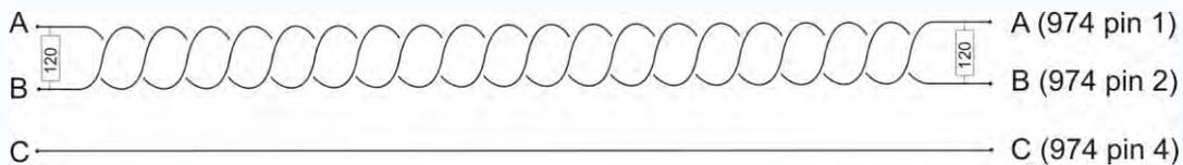
*RS485 twisted pair cable run with 120 Ω terminator resistors (974B with 15 pin connector)*
