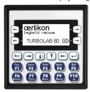
By pressing the pushbutton within 15 seconds, the default settings of the system can be changed, see Chapter 3.3.
