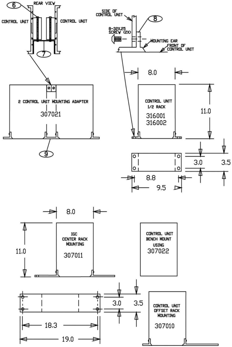
Figure 1-3 Mounting Configurations
