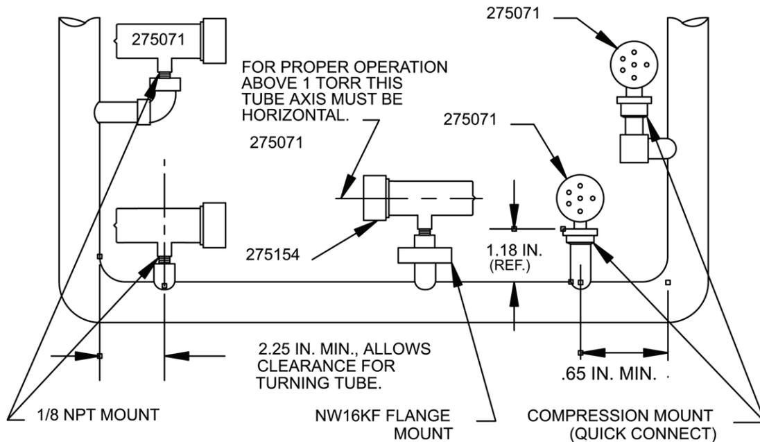
Figure 2-2 Convectron Gauge Mounting Clearances
