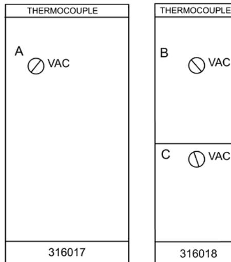
Figure 3-4 Thermocouple Gauge Modules, Front Panel
