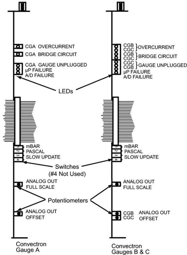
Figure 2-12 Convectron Modules, Top View (Controller Cover Removed)
