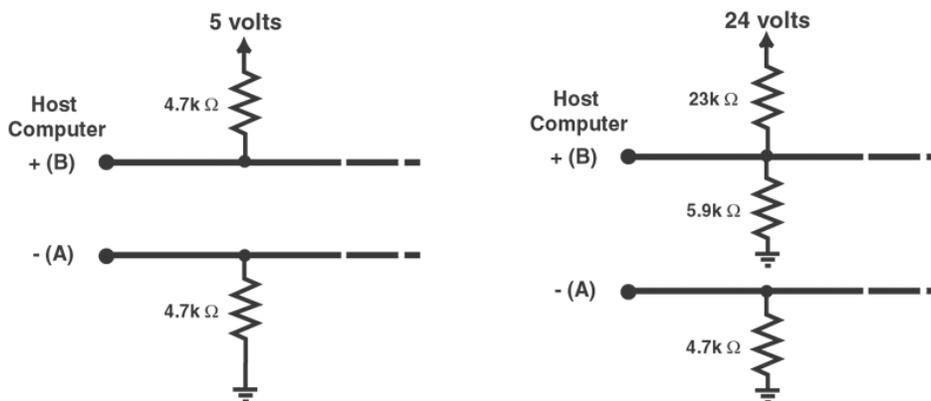
Figure 8-3 RS-485 Bias Resistors
