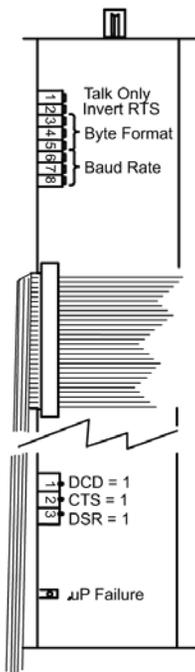
Figure 6-2 RS-232 Module, Top View (Controller Cover Removed)
