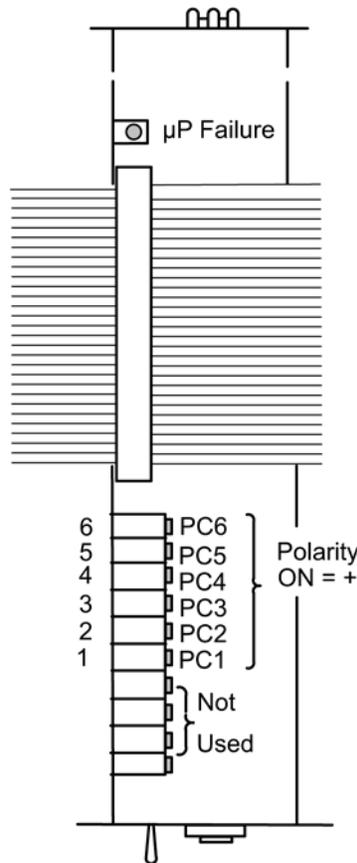
Figure 5-4 Process Control Module, Top View (Controller Cover Removed)
