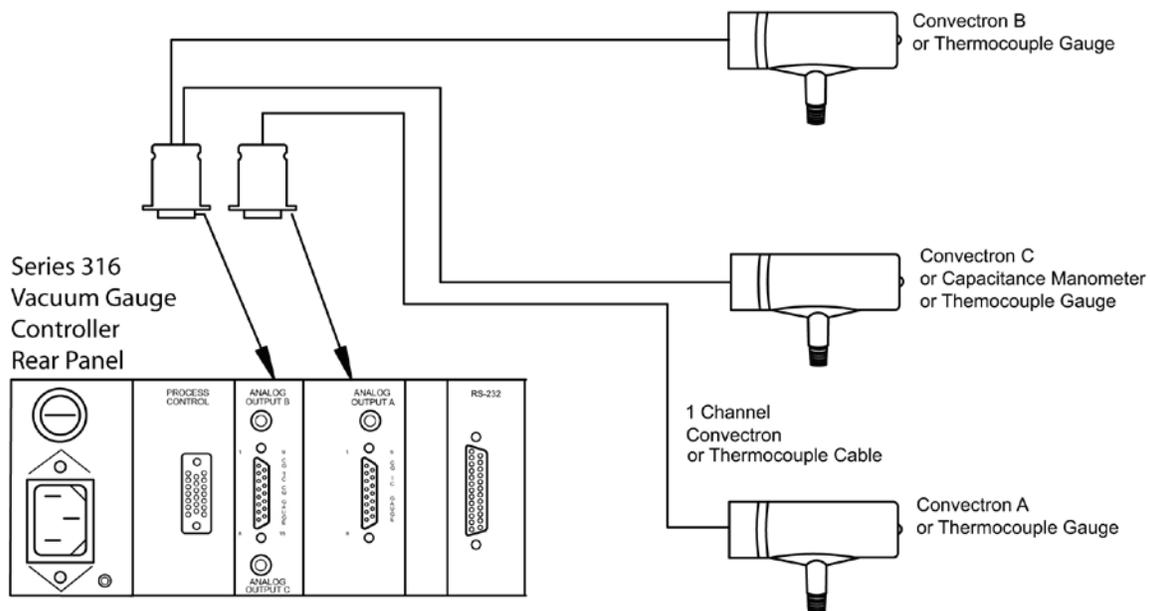
Figure 1-4 Cable Connections
