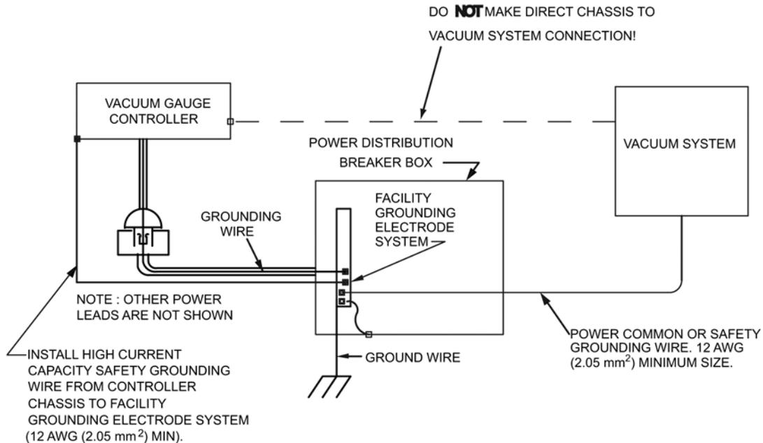
Figure 1-5 Correct System Grounding
