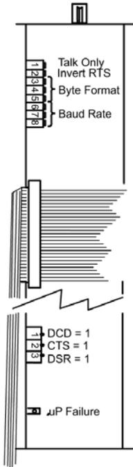
Figure 6-1 RS-232 Module, Top View (Controller Cover Removed)
