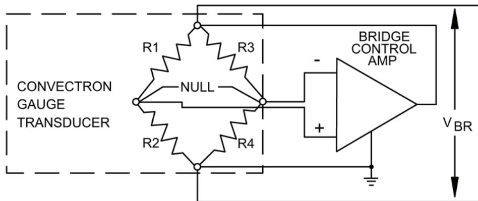
Figure 2- 13 Simplified Schematic of the Convector Gauge
