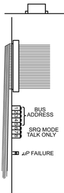
Figure 7-1 IEEE 488 Module, Top View (Controller Cover Removed)
