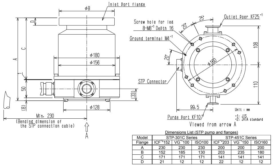
Figure 13.2 External Appearance of the STP Pump [Chemical Specific Type C] (Example: STP-301C)
