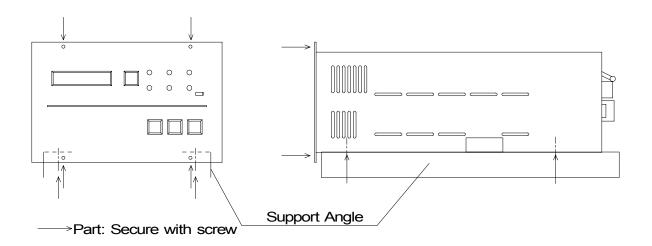
Figure 6.6 Example of Securing the STP Control Unit
