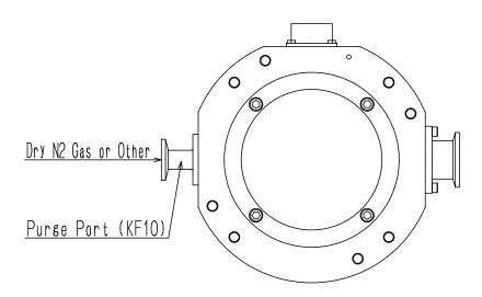
Figure 4.8 Connecting the Purge Port
