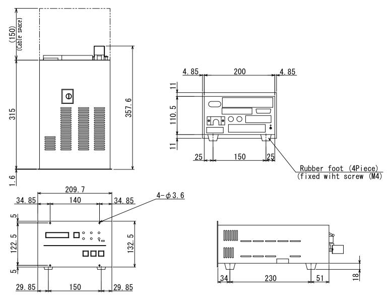
Figure 13.4 External Appearance of the the STP Control Unit
