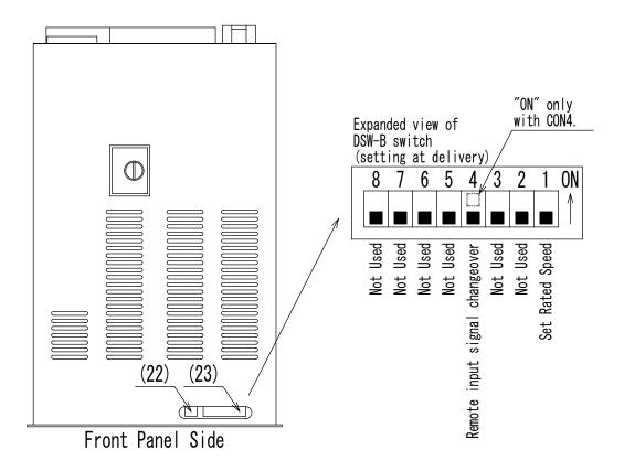
Figure 6.3 STP Control Unit Top Panel
