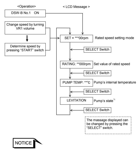
♦ The rated speed returns to 48,000 rpm (initial setting) by setting dip switch 1 of DSW-B to "OFF".
