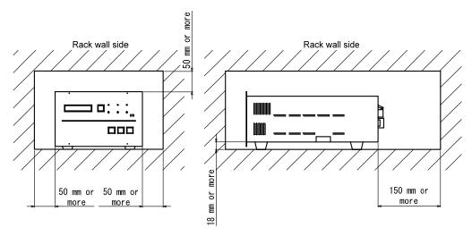
Figure 6.5 Peripheral Spaces of the STP Control Unit
