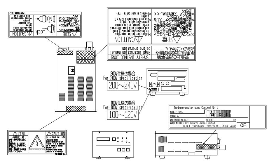
Figure 13.5 Label Affixing Positions for the STP Control Unit
