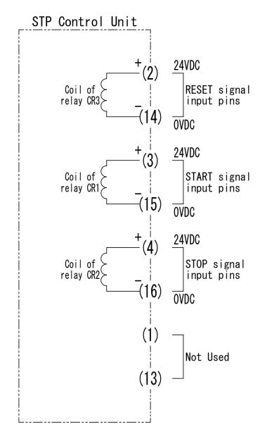
Figure 8.3 CON4 Remote Input Signal Connector
