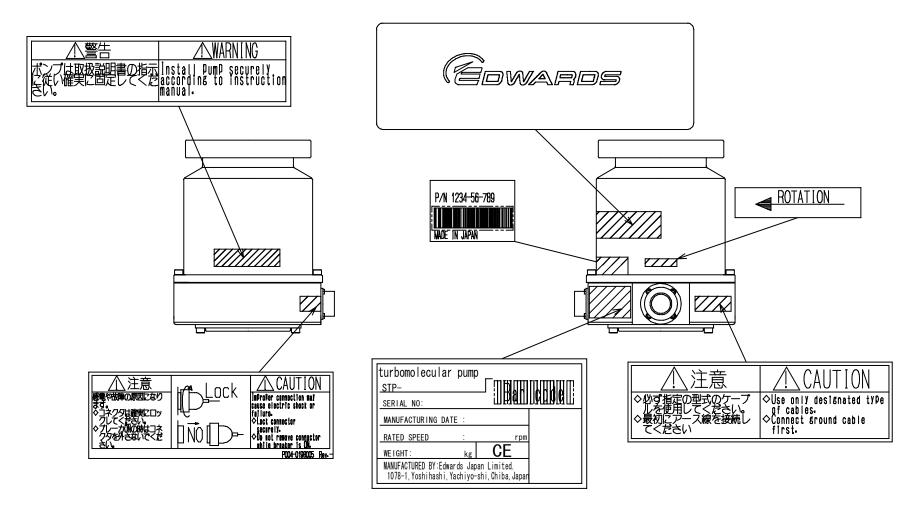
Figure 13.3 Label Affixing Position for the STP Pump
