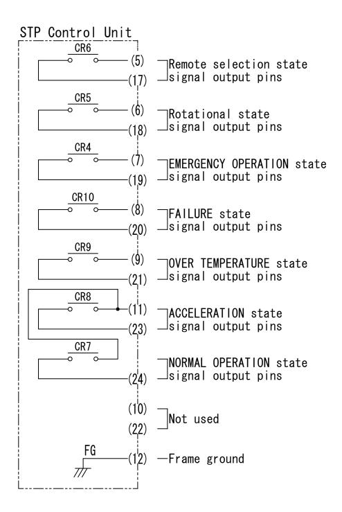
Figure 8.4 CON4 Remote Output Signal Connector
