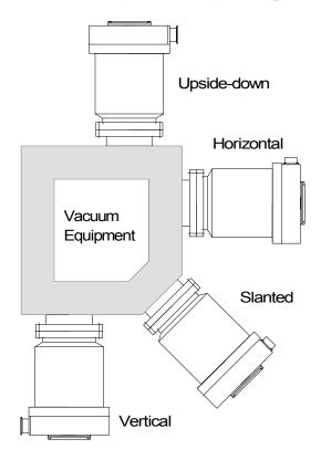
Figure 4.3 STP Pump Installation Positions
