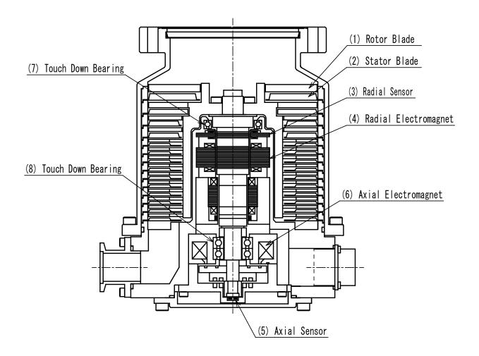
Figure 2.1 Cross Sectional View of the STP Pump
