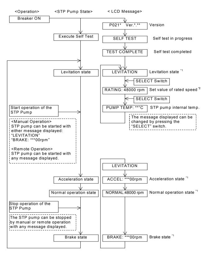
Figure 7.1 STP Pump Operation Procedures
