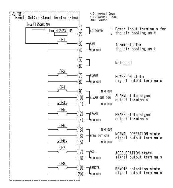
Figure 8.1 I/O TB1 Remote Output Signal Terminal Block
