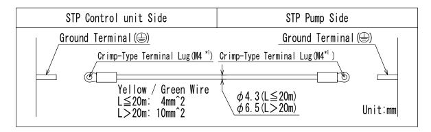
Figure 6.7 External Dimensions of Ground Cable
