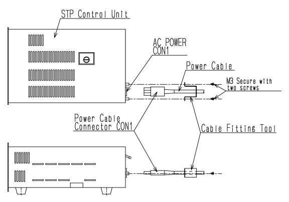
Figure 6.11 How to Secure the Power Cable
