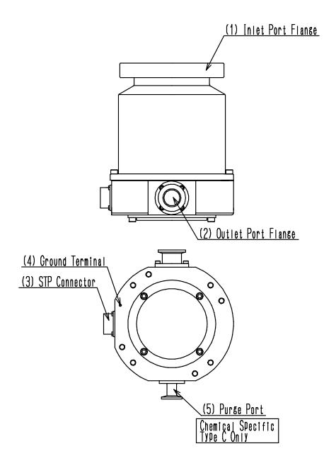
Figure 4.1 Configuration of the STP Pump
