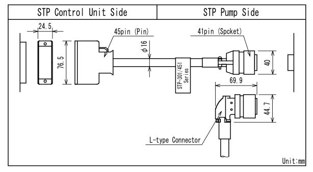
Figure 6.8 External Dimensions of STP Connection Cable
