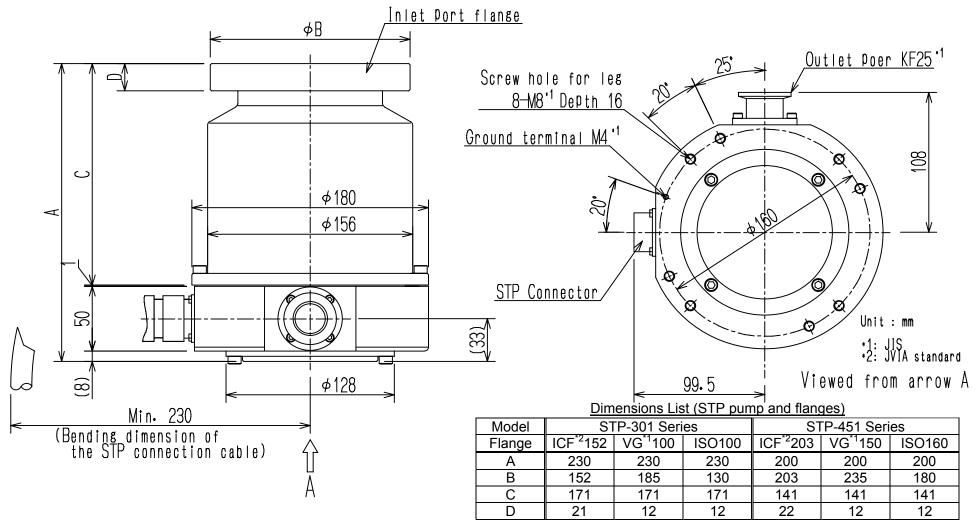
Figure 13.1 External Appearance of the STP Pump [without Anti-Corrosion Treatment] (Example: STP-301)
