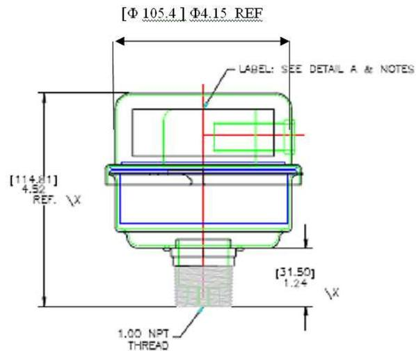
**Figure 1-6 Exhaust/Resonator Dimensions**
