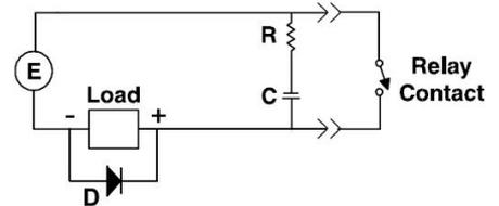
Note that  $R_{min} = 0.5 \Omega$  and  $C_{min} = 1 \times 10E-9$  F, D is a fast transient suppression diode.
