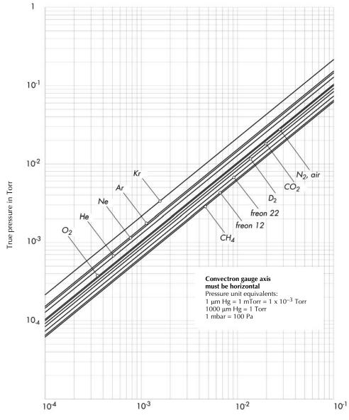
Figure 5-1 Reading true pressure values,  $10^{-4}$  to  $10^{-1}$  Torr
