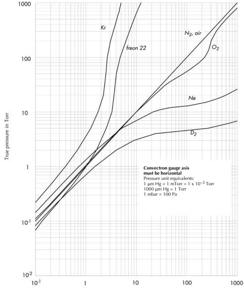
Figure 5-3 Reading true pressure values,  $10^{-1}$  to 1000 Torr
