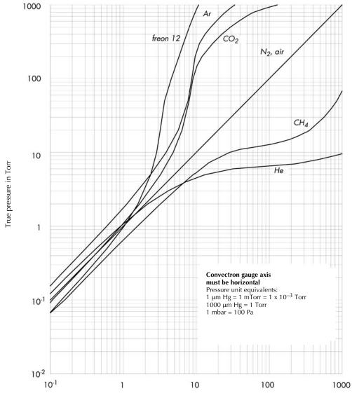
Figure 5-2 Reading true pressure values, 10<sup>-1</sup> to 1000 Torr
