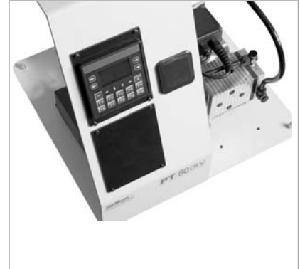
Control unit installed in the PT 80 Dry pump system
