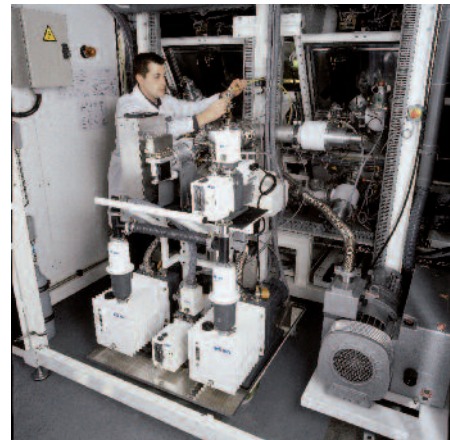
Pumping unit integrated in an industrial Leak Detection System
