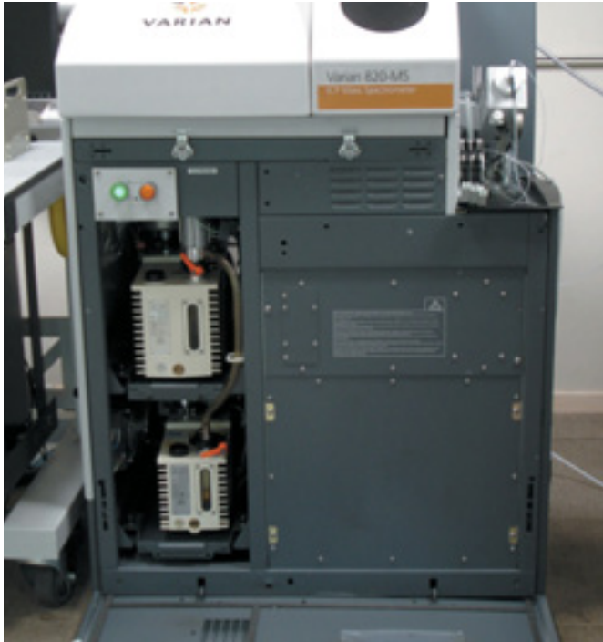
ICP-MS. Photo courtesy Varian Scientific Instruments.
