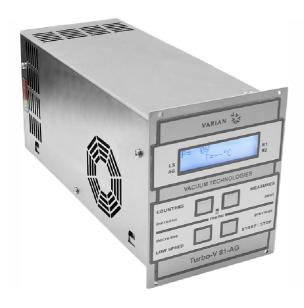
The Turbo-V 81-AG Rack controller is a microprocessor-controlled frequency converter with new, enhanced features that allow greater control and communication capabilities. This compact, 1/4 rack unit is designed for full worldwide compatibility, for vent valve control, active gauge pressure reading and pump operation parameters control, as well as for self diagnostic and protection features.
