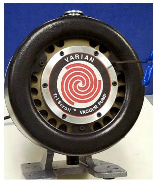
7. Install cowling over pump module. Secure with three M5x16 screws.
