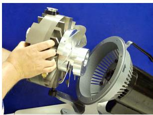
5. Install pump module on frame, aligning fingers on fan assembly with fingers on coupling. Assure proper fit of dowel pins on mating holes in frame.
