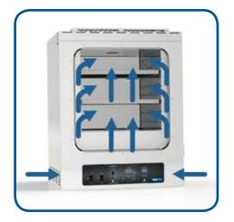
SHEL LAB gravity ovens rely on the natural thermal properties of heating - warm air rises. We utilize this airflow and combine it with our unique air duct system to allow heated air to move up through these ducts improving uniformity. Gravity ovens are commonly used in applications when natural heating is required without the assistance of fans or blowers. This technology is ideal for applications which include samples that are sensitive to air movement.
