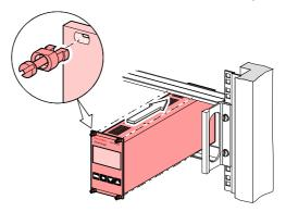
... and fasten the adapter panel to the rack chassis adapter using the screws supplied with the TPG 262.
