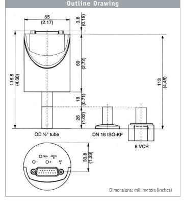
The Varian CDG-500 series of temperature compensated Capacitance Diaphragm gauges provides a high level of accuracy in the high pressure region. Full scale measurement ranges are available from 1000 Torr to 1 Torr. The CDG-500 series uses a corrosion resistant ultra pure alumina ceramic diaphragm providing exceptional signal stability, fast recovery from atmosphere, short warm-up times and unparalleled robustness.
