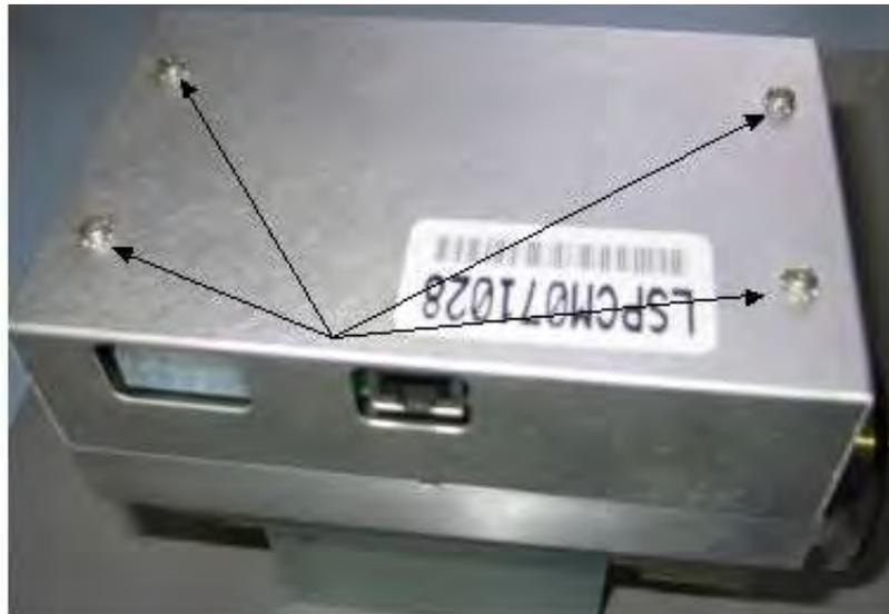
**Figure B-50 Spectrometer Cover Screws**
