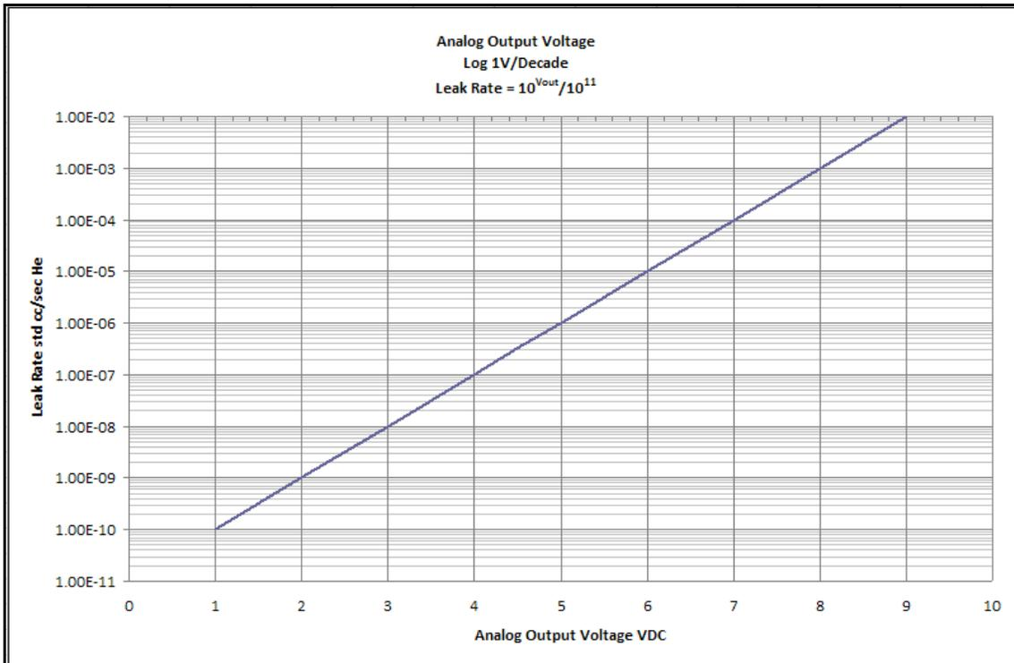
**Figure 3-3 Leak Rate vs Analog Output - 1VDec**
