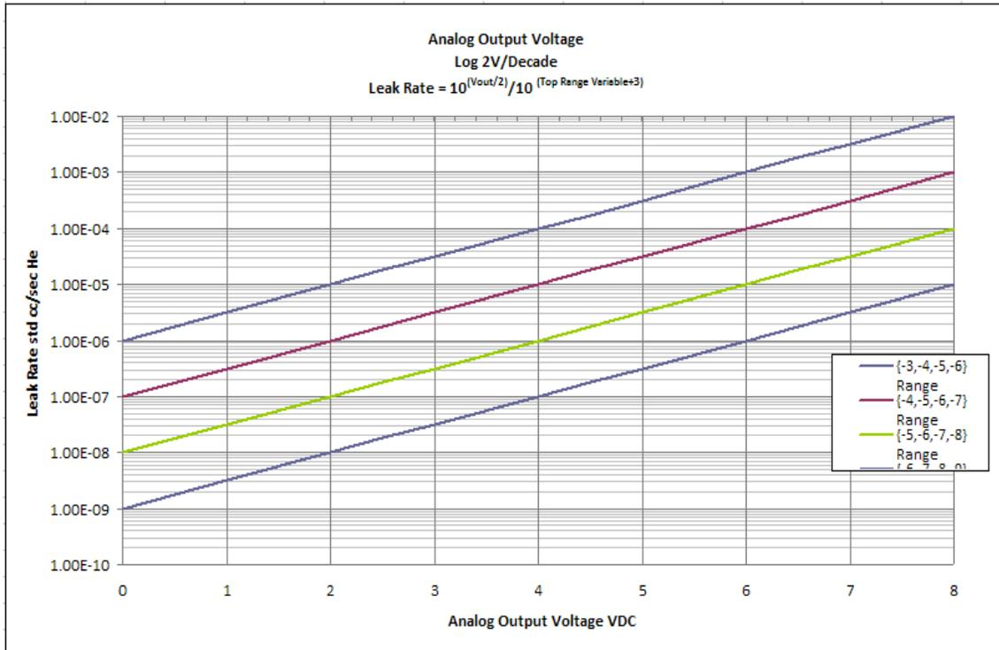
**Figure 3-4 Leak Rate vs Analog Output - 2V/Dec**
