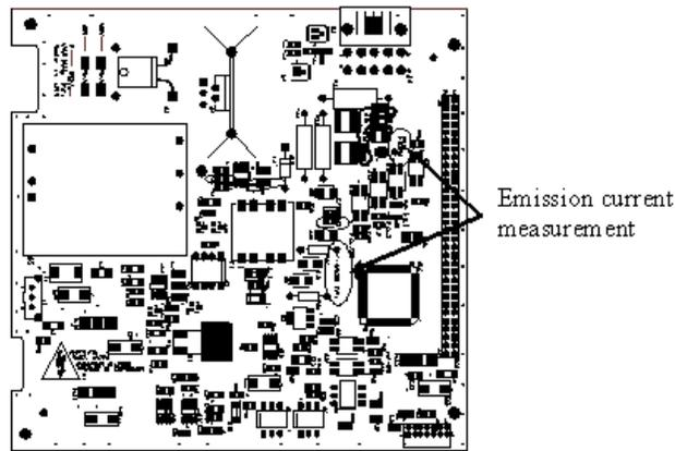
**Figure C-4 Ion Source Board - Measurement Points**
