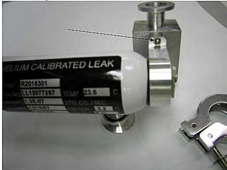
**Figure B-44 Calibrated Leak Screws**
