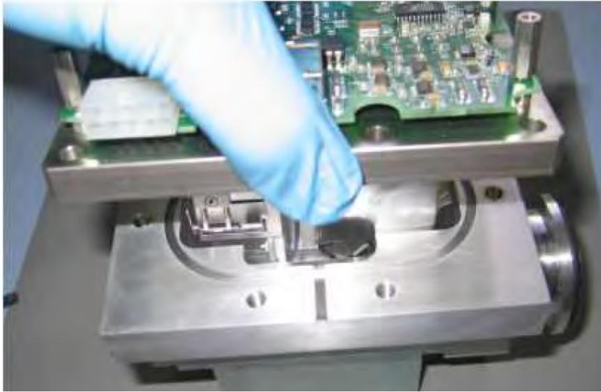
**Figure B-80 Spectrometer Assembly Removal**
