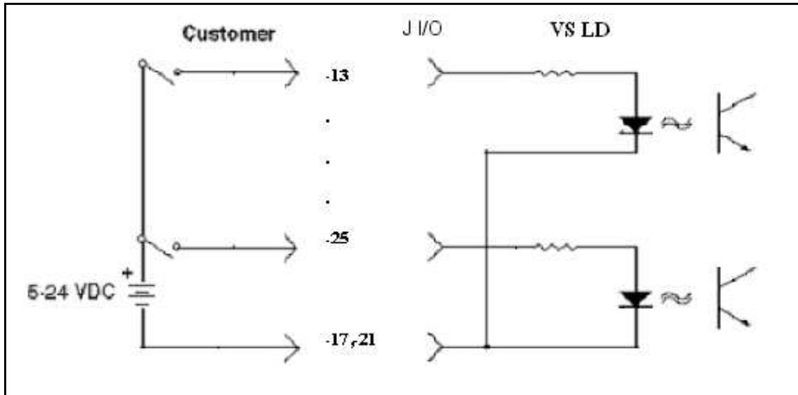
Figure 3-2 Optically Isolated Input Circuit Sketch
