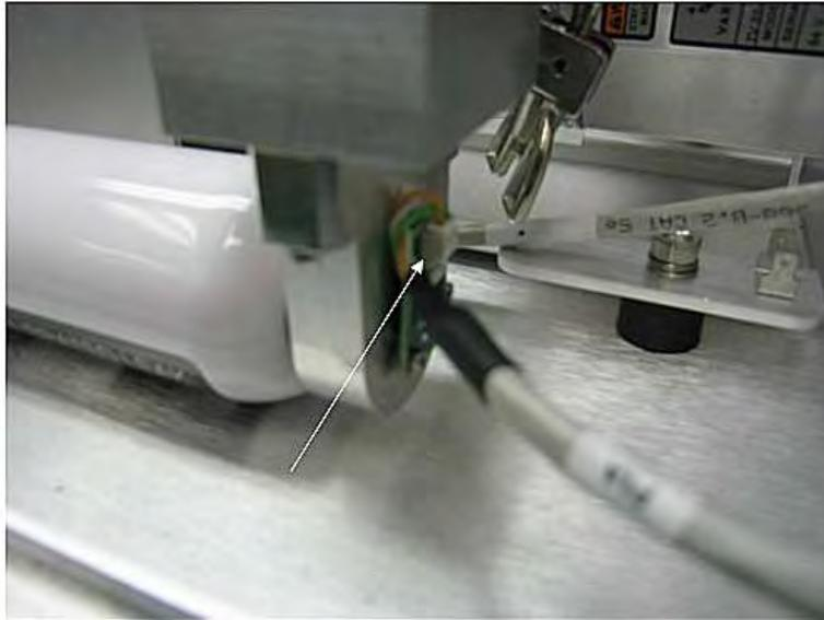
**Figure B-42 Cable to Calibrated Leak Connection**
