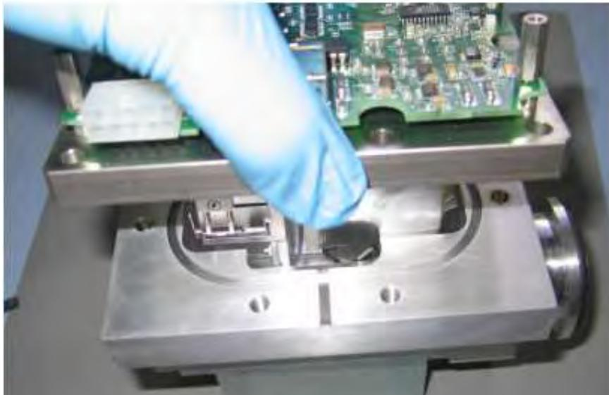
**Figure B-63 Spectrometer Assembly Removal**
