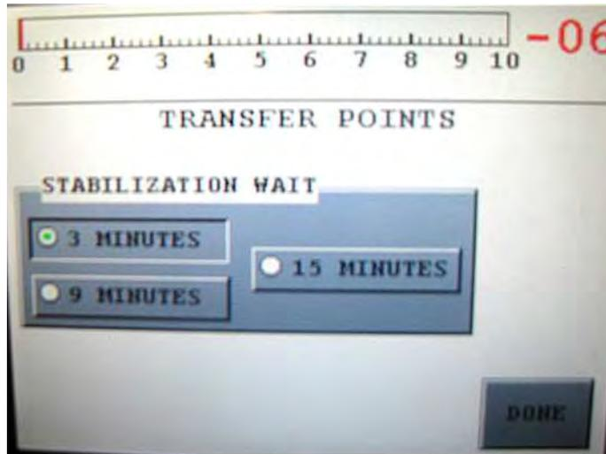
**Figure 2-9 Transfer Points with Stabilization Wait Timer**
