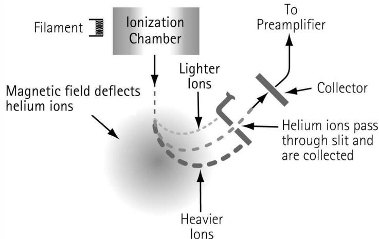
**Figure D-1 Magnetic Separation Principle**
