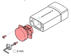
Place the new sensor without twisting it and lock it with the screws.
