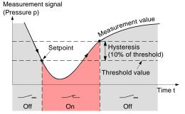
The setpoints SP1 and SP2 are factory set to the lower measurement range limit and therefore do not switch.
