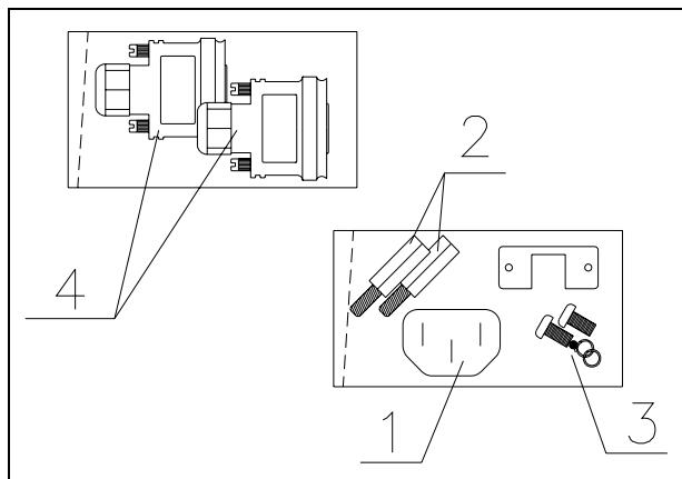
1. Remove the spring bracket mounted on standard IEC socket.
