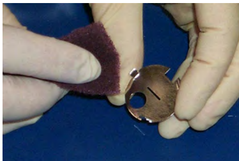
Figure 4-20 Discolored Ground Slit Plate
