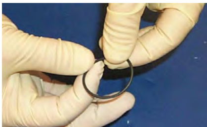
Figure 4-23 Inspecting the O-ring
