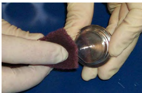
Figure 4-21 Discolored Ground Magnet Pole Piece
