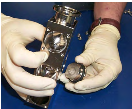
Figure 4-19 Removing the Second Magnetic Pole Piece
