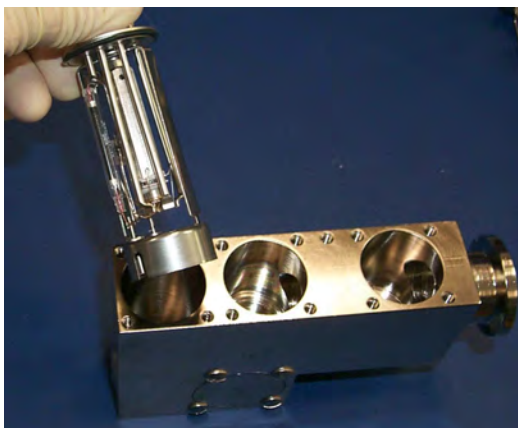
Figure 4-16 Removing the Preamplifier
