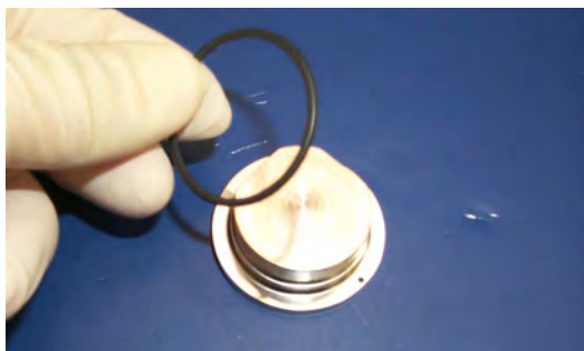
Figure 4-18 Removing the O-ring from Magnetic Pole Piece
