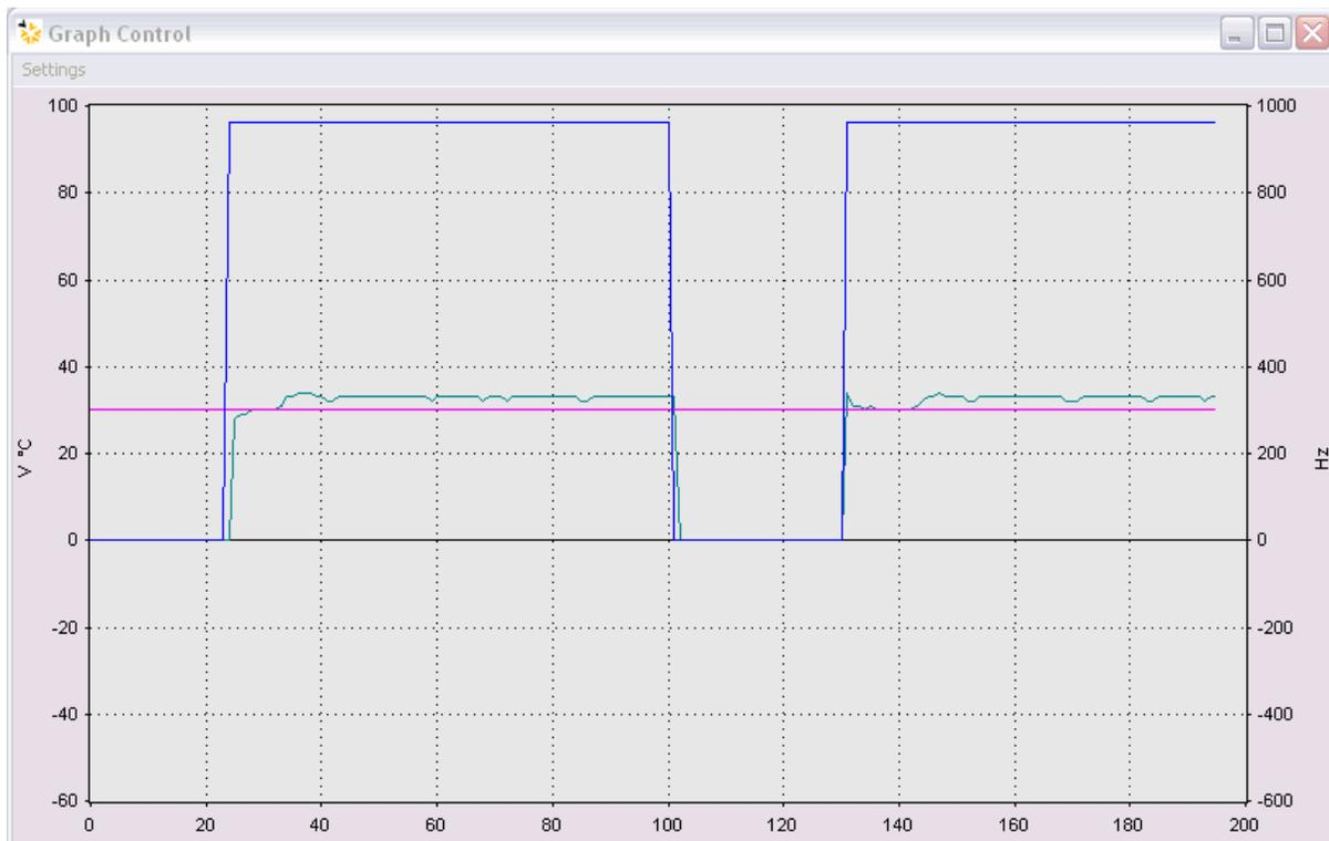
The Graph window plots till 8 different tracks allocable on two different Y axes and continuously shows their timing trend on the screen. You can add new fields right-clicking on the window list in the Single Pump Control Panel Window. The Graph window is completely sizable and it has axes limits completely configurable. Moreover for each track you can choose colour and Y axis (primary or secondary).
