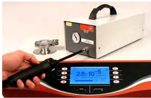
Fig. 6-81 Sniffing external test leak
