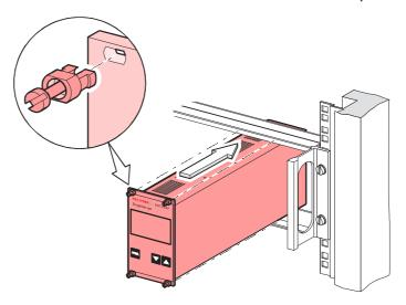
... and fasten the adapter panel to the rack chassis adapter using the screws supplied with the TPG 261.
