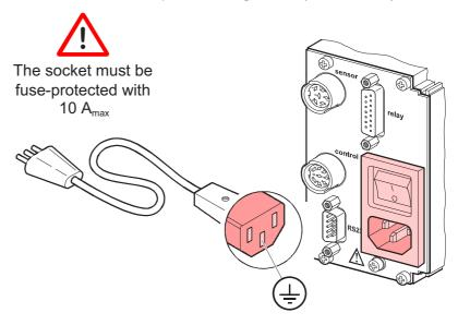
If the unit is installed in a switching cabinet, the mains voltage should be supplied and turned on via a central distributor.
