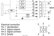
Pin 5 Supply common (GND) Pin 6 Screen Connector soldering side
