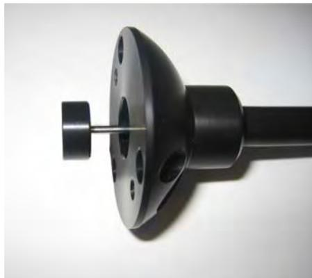
Take out the capillary and remove the taper gasket at the top of the sniffer tip.
