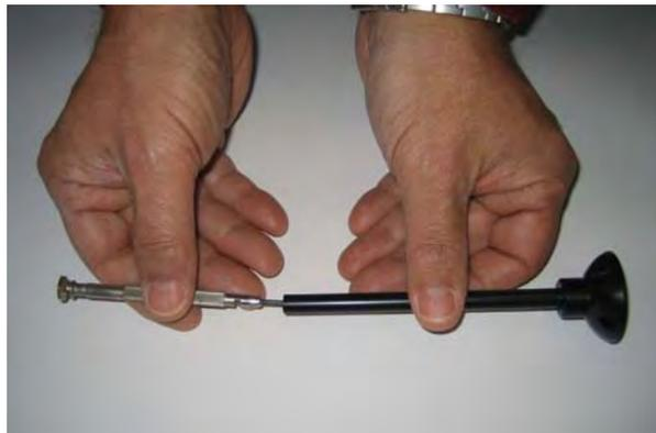
Take a small pin or needle (about Ø 0.5 mm) and press the capillary from the top out off the tip (Fig. 10-76). Then the taper gasket (Fig. 10-73,3) at the tip can drop out.
