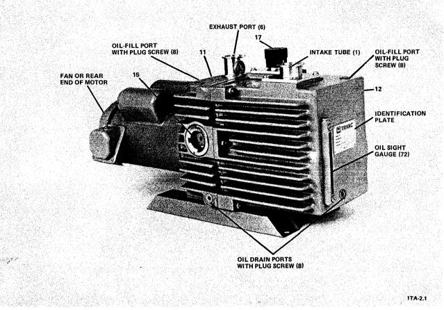
Figure 1-1. Location of the Identification Plate, the Oil Fill Ports and the Oil Drain Ports (D30A Pump Model Shown).
