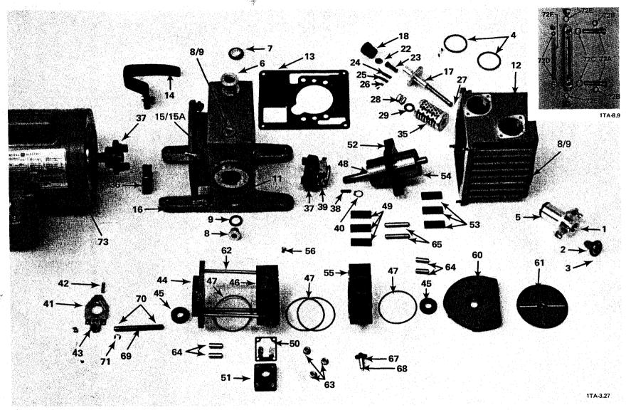
Figure 7-1. Disassembled Pump (D2A Pump Model Shown)
