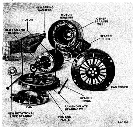
Figure 5-17. Disassembled Motor (D30A Motor Shown)
