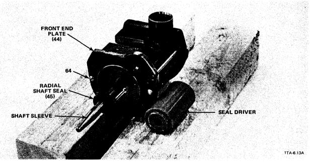
Figure 5-22. Using a Shaft Sleeve to Install the Radial Shaft Seal into the Front End Plate (D2A Pump Model Shown) Step F-6 k (Cont'd.)
