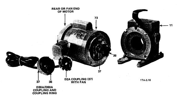
Figure 5-15. Coupling Housing and Motor (D2A Pump Model Shown)
