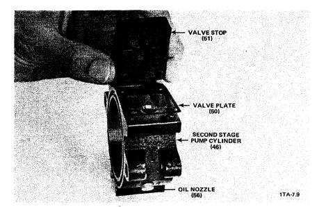
NOTE: The valve plate (50) on the D30A/D60A/D90A pump models has four tabs rather than two. Figure 5-14. Removing the Valve Stop and Plate (D2A Pump Model Shown)
