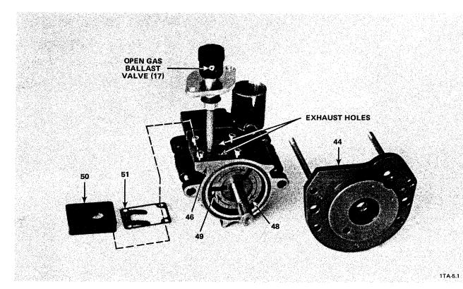
NOTE: This photograph is for illustration purposes only. When assembled, the cap end of the gas ballast valve (17) is attached outside the top of the oil casing (12) (see Figure 1-1), and an oil filter (35) and other parts fit around the valve (17) stem (see Figure 5-10B).
