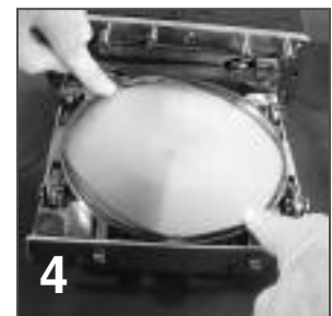
Continue pressing O-ring into groove at 180°-apart intervals.
