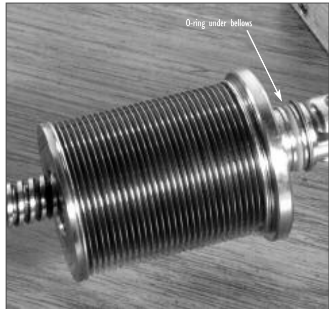
Twist the bellows slightly to pull free of the O-ring
