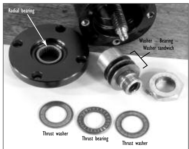
Drive nut and bearing block assembly parts
