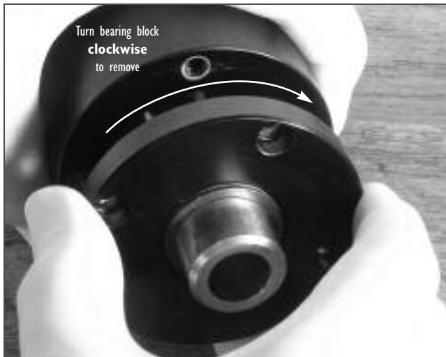
ACME thread on actuator stem is left-handed
