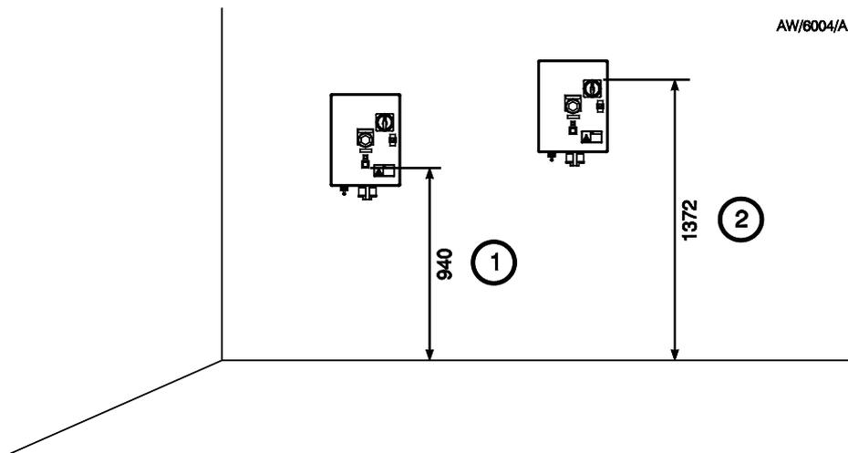
1. Minimum mount height to bottom of reset push button
