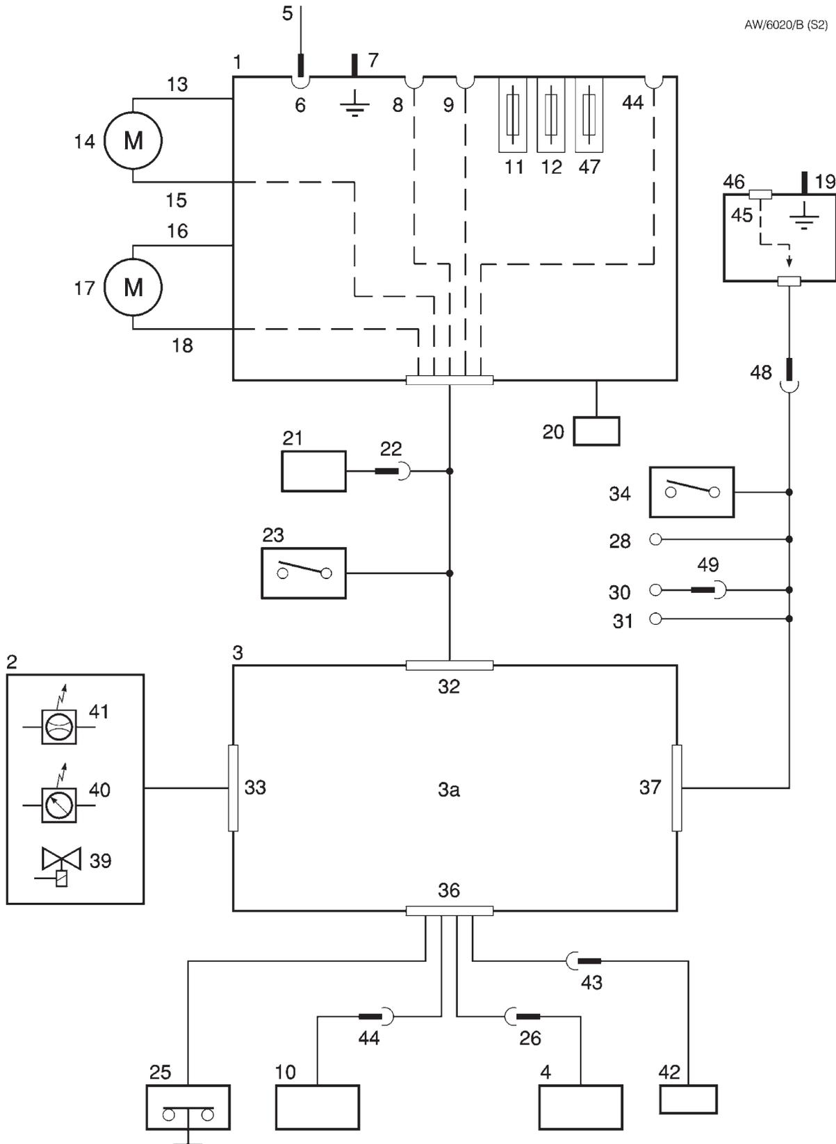
Figure 1-3 - Schematic diagram of the iH80/iH600 electrical systems
