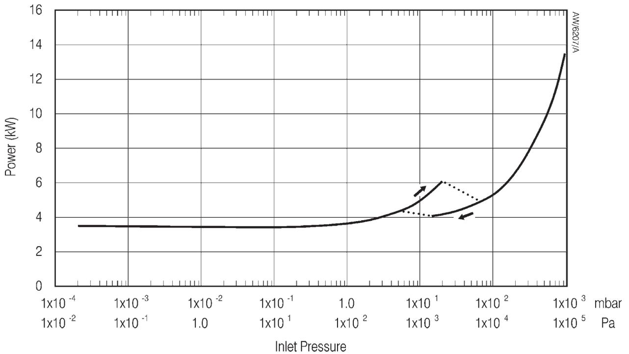
Note: Discontinuity in curves are as a result of the HCMB pressure relief valve opening and closing
