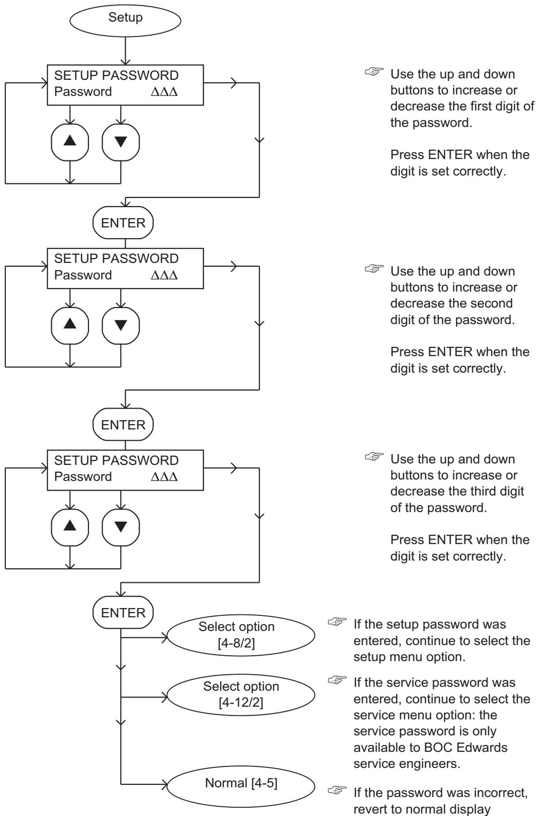
Figure 4-8 - Setup menu: sheet 1 of 3
