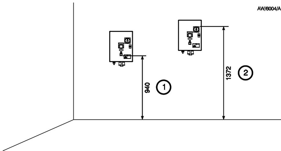
1. Minimum mount height to bottom of reset push button
