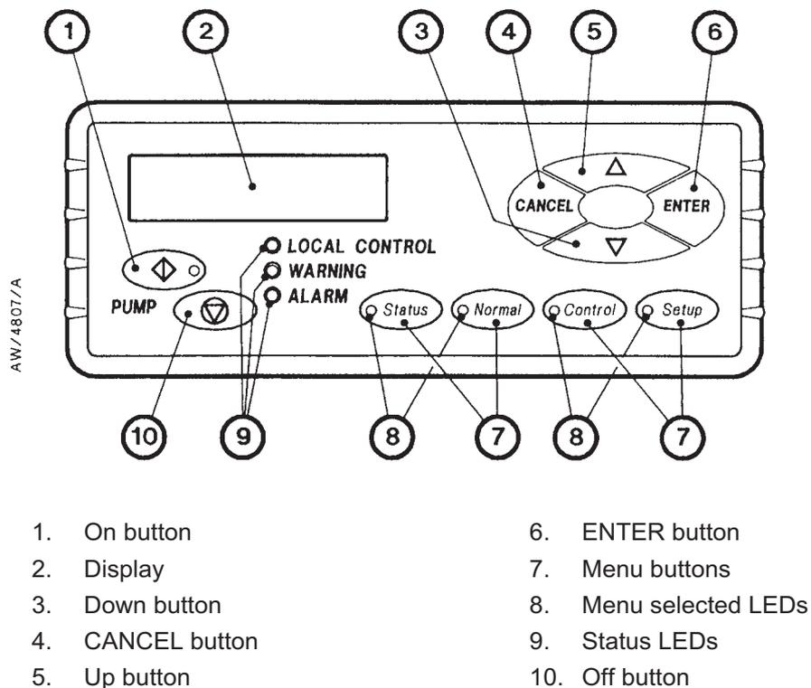
Figure 1-8 - Front panel of the pump display terminal
