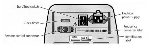
■ Electrical frequency converter is in accordance with CE standards and offers the following voltage range:
